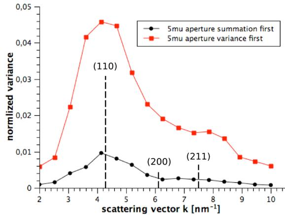
**Figure 3.** Plot of the normalized variance  $V(k)$  of the intensity of images taken with a 5  $\mu\text{m}$  objective aperture. The two curves differ by the method of averaging over the angle  $\phi$ . Lower values of  $V(k)$  are obtained by calculating  $V$  of images summed first over  $\phi$ . The position of structure factors  $(hkl)$  of B2 ordered CuZr is indicated.
