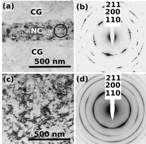
Figure 1. TEM study of the nanocrystalline (NC) structures occurring in HPT-deformed FeAl as a function of shear strain  $\gamma$ . (a)  $\gamma=1200\%$ ; bright-field (BF) image showing a band containing NC material embedded in coarse-grained (CG) material. (b) SAD of the area indicated in (a). (c) At  $\gamma>7100\%$  the sample is homogeneously NC. (d) SAD of (c).
