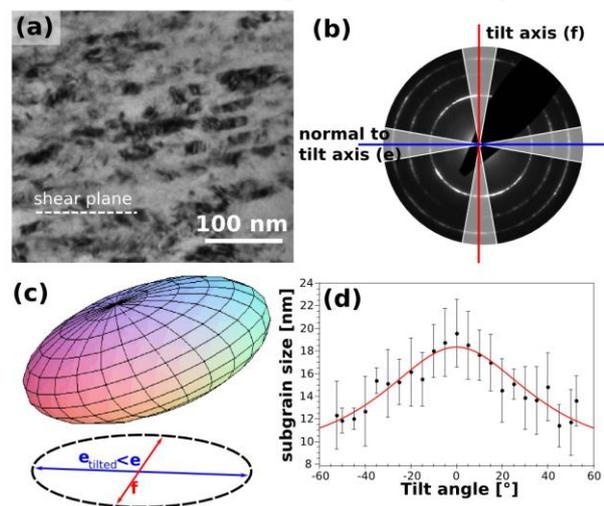
Figure 2. (a) Cross section image showing elongated grains. (b-d) To study the elongation of the crystallites from a top-view sample a large number of SAD patterns was recorded and the size of the platelet shaped crystallites was evaluated in the direction  $e+f$  for various tilt angle. When tilting the sample, the size measured in direction  $e$  decreases allowing to calculate the elongation.
