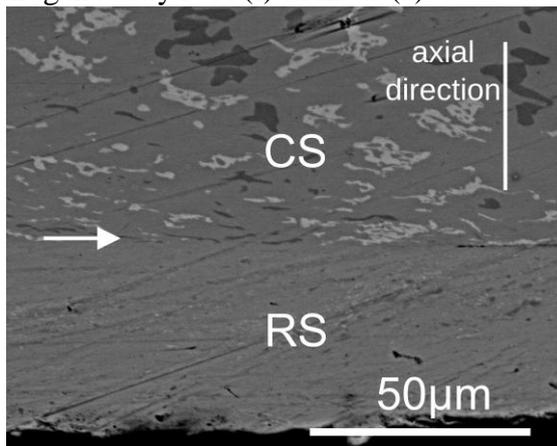
Figure 3. Cross section SEM image of a HPT disk deformed 10 turns. Different regions are clearly distinguishable and separated by a sharp line (marked by arrow): a coarse crystalline structure (CS) with different phases and a region with homogeneous contrast indicating that the structure is refined (RS).
