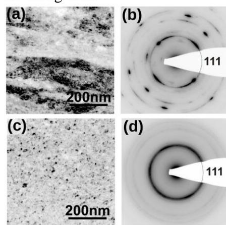
Figure 4. Cross section dark field images of the HPT disk shown in Figure 3 (N.B. black/white inverted for better visibility). (a) is taken from the coarse crystalline region and (c) from the refined structure. The grain size decreases from  $>1 \mu\text{m}$  to  $<10 \text{ nm}$  within a few  $\mu\text{m}$ .
