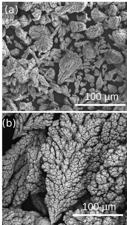
**Figure 2.** SEM images of NiCoFe powder deposited at  $j=1 \text{ A cm}^{-2}$  after (a) 180 s and (b) 1800 s deposition time. The images reveal that with increasing deposition time the particle size increases by a factor of about 10. The particles show a 3D dendritic morphology.
