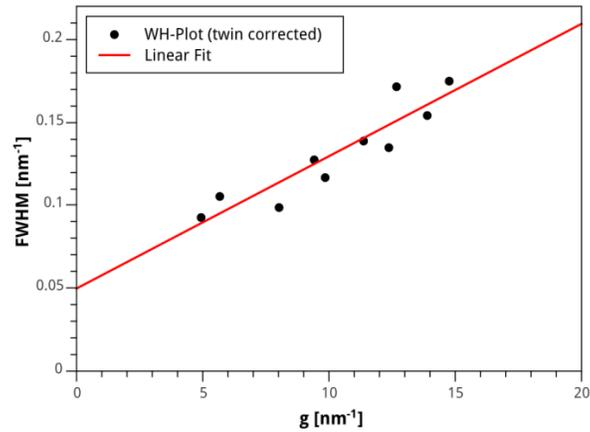
**Figure 6.** Williamson-Hall plot from the electron diffraction images of electrodeposited NiCoFe powders ( $j=1 \text{ A cm}^{-2}$ , deposition time=180 s). The full width half maximum (FWHM) values plotted as a function of the reciprocal vector  $g$  are corrected for the presence of twins according to ref [24], allowing to determine the density of the twins.
