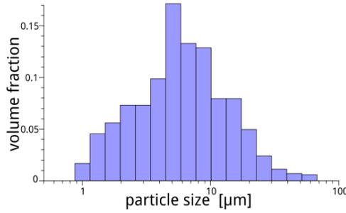
**Figure 3.** Particle size distribution of NiCoFe alloy powders ( $j=1 \text{ A cm}^{-2}$ , deposition time,  $t=180 \text{ s}$ ) measured by the sedimentation method. The distribution shows a mean of  $10 \mu\text{m}$ .
