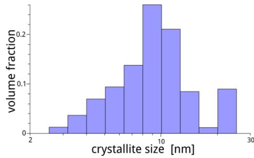
**Figure 5.** Crystallite size distribution of the NiCoFe powder ( $j=1 \text{ A cm}^{-2}$ , deposition time=180 s), determined from the contrast of the crystallites in TEM dark-field images. The distribution shows a volume weighted mean of  $10 \pm 1 \text{ nm}$ .
