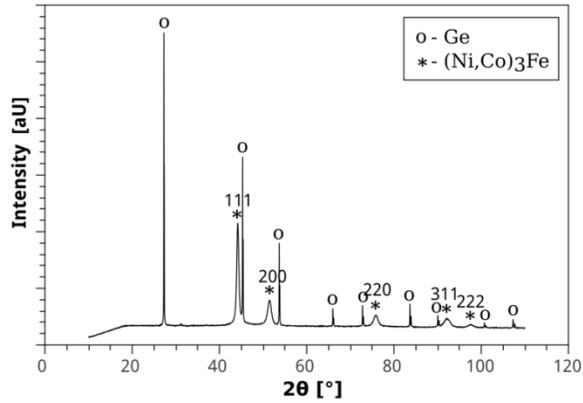
**Figure 1.** X-ray profile of the electrodeposited NiCoFe powder obtained at a current density of  $j=1 \text{ A cm}^{-2}$  and after 180s showing broad peaks. The sharp peaks correspond to the Ge standard, that was added to allow a precise determination of the lattice constant.
